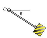
Determine the mass moment of inertia with respect to *O*.
